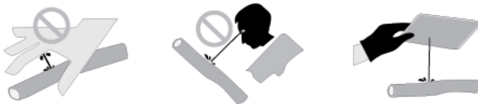
Figure 1-5 Prevent burns from high pressure oil
