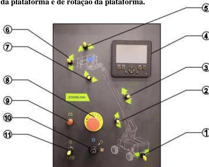
Figure 2-2 Painel de Controle no Solo
