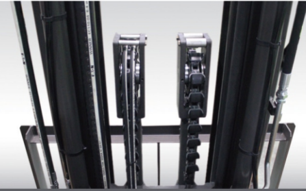
Mast triple full free equipped with double front cylinder, increasing greatly the driver operating field of vision.
