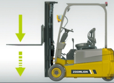
Mast intelligent buffer system, when the fork falls to the ground, the descent speed will be automatically reduced to prevent the damage to the goods from impact of vehicle.
