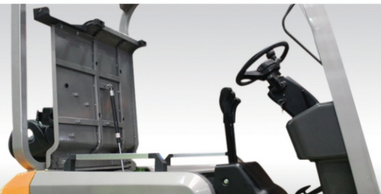
The battery cover adopts hydraulic tappet support, it can be fully opened, easy to maintain the battery.
