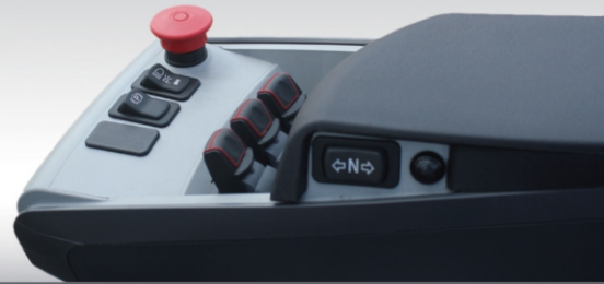
optional Fingertip control system set to rise and fall, forward, backward, lateral and emergency stop switch, a horn, lighting control and other control buttons in one.
